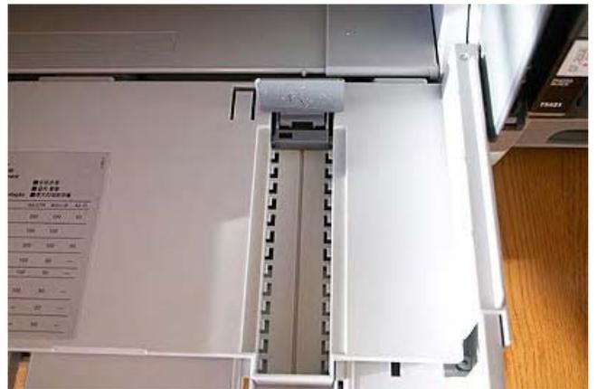
The paper tray stopper in the paper tray area, shown at its furthest and closest reach, depending on the paper size used. Below the paper push down lever, whose function is to press on the stack of paper in the tray
