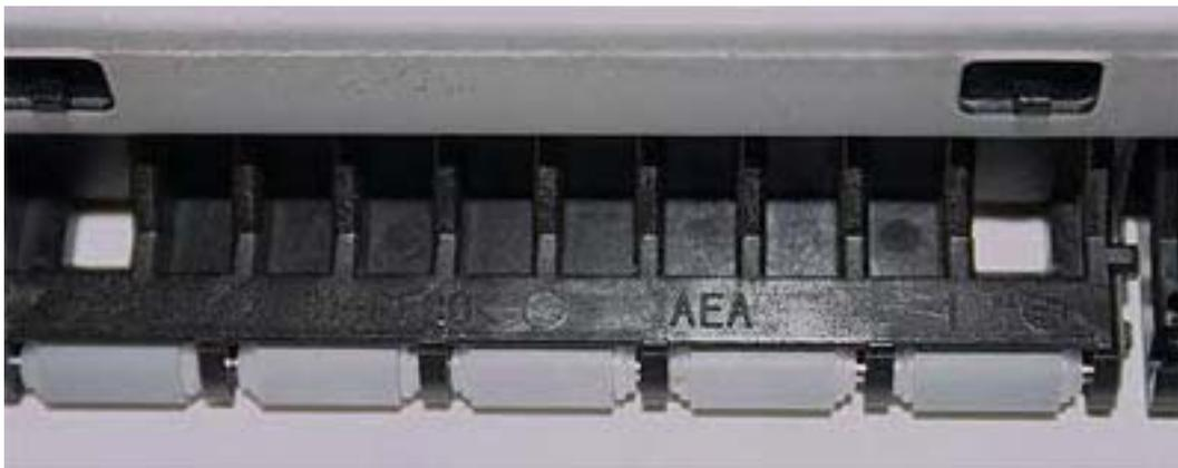
The smooth plastic rollers that push down on the paper as it comes out of the printer. On the first Epson printers, such as the 3000, those rollers had teeth instead of a smooth rubberized cover and were referred to as pizza wheels. I removed them from my printers to avoid damage to the paper. Interestingly, not having them made no difference whatsoever to printer operation. I just had to make sure to put them back in when sending the printer for service or when I eventually sold it.
